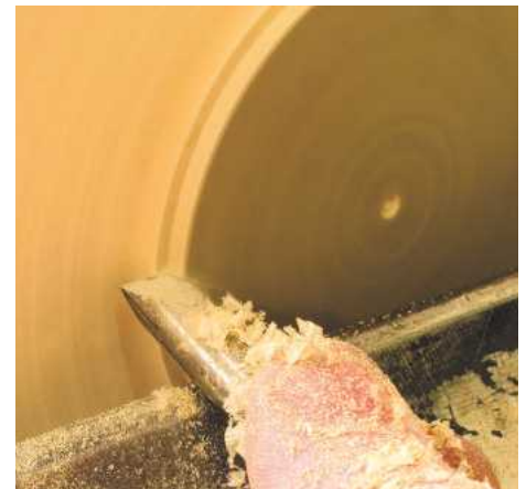
▲ Pic.6 The 10mm round skew is used to turn the foot, and will also create a small flat alongside the foot that will sit against the top of the jaws for strength and accuracy
